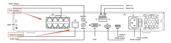
As shown in the above picture, a PoE NVR has 2 NICs (External Ethernet NIC and Internal PoE NIC). Both NICs can be connected with cameras. There are 2 different methods to add all 16 cameras.
